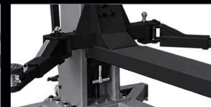
Rear support arms adjust to the vehicle's lift points.
