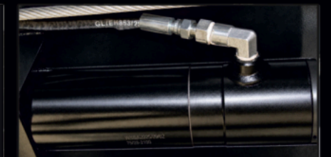
Hydraulic cylinder and protective fitting.
