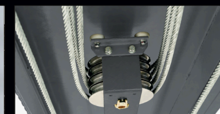
A hydraulic cylinder and pulleys drive the platform.
