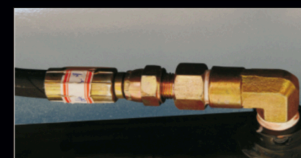
A line-break valve helps limit sudden hydraulic descent.
