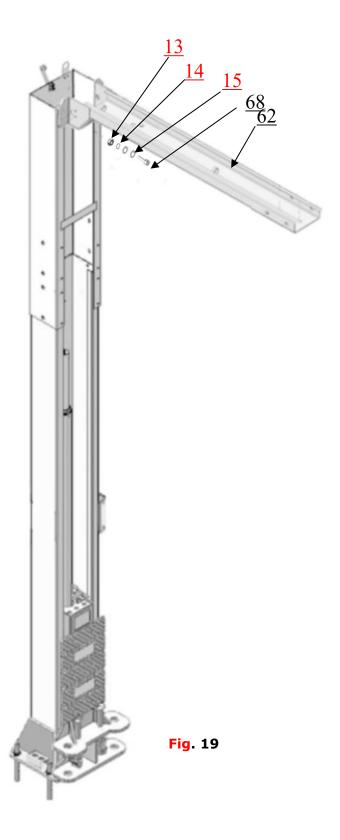
2. Assemble overhead top beam, tighten the columns anchor bolts (See Fig. 20).
