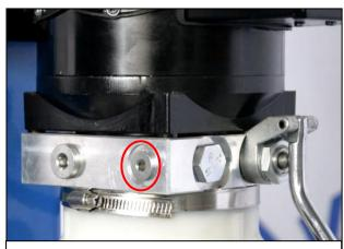
D. Assemble the hex plug by Step A to this left oil inlet port.
