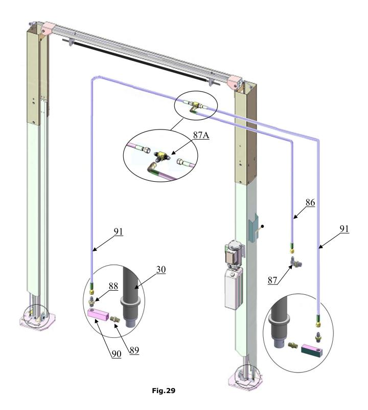
Tighten all the hydraulic fittings, and fill the reservoir with hydraulic oil.
