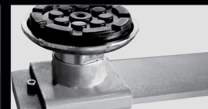
Rubber pads and height adapters contact the lift points.
