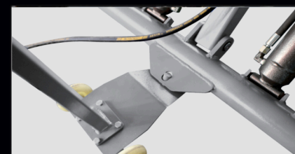
The trolley connection helps move the unloaded lift.
