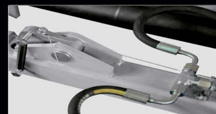
The mechanical safety system supports the raised platform.
