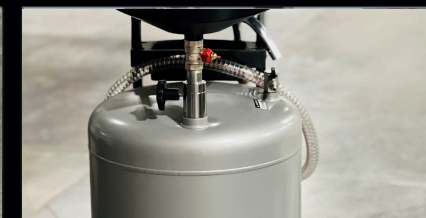
Discharge hose and tank fittings.
