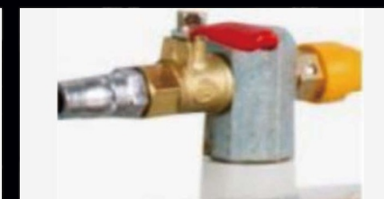
Shop-air evacuation connection.
