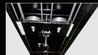
Pulley and cable under upper main platform
