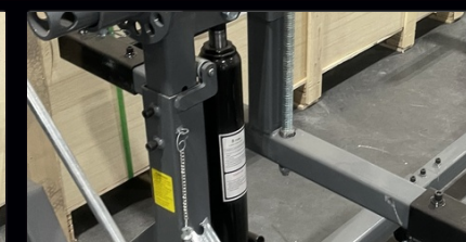
Hydraulic jack and lifting upright.
