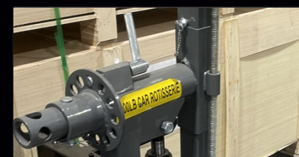
Hand-cranked rotation gearbox.
