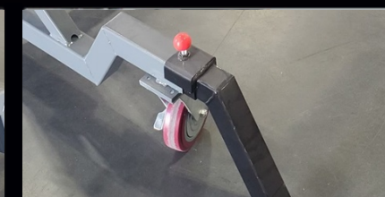
Locking caster and stabilizer foot.
